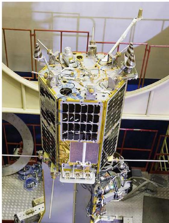
This is the third satellite created by the specialists of ISS-Reshetnev and is based on the Yubileyniy platform, which features a hexagonal prism structure with body-mounted solar cells. It was launched into orbit last December 26 from the Plesetsk Cosmodrome and is in an elliptical orbit with a perigee of 1,175 kilometers (729 miles), an apogee of 1,511 kilometers (937 miles), and an inclination of 82.5°. Transmitter power is 5 W, and the beacon is on 435.605 MHz (identifying as RS-44).
