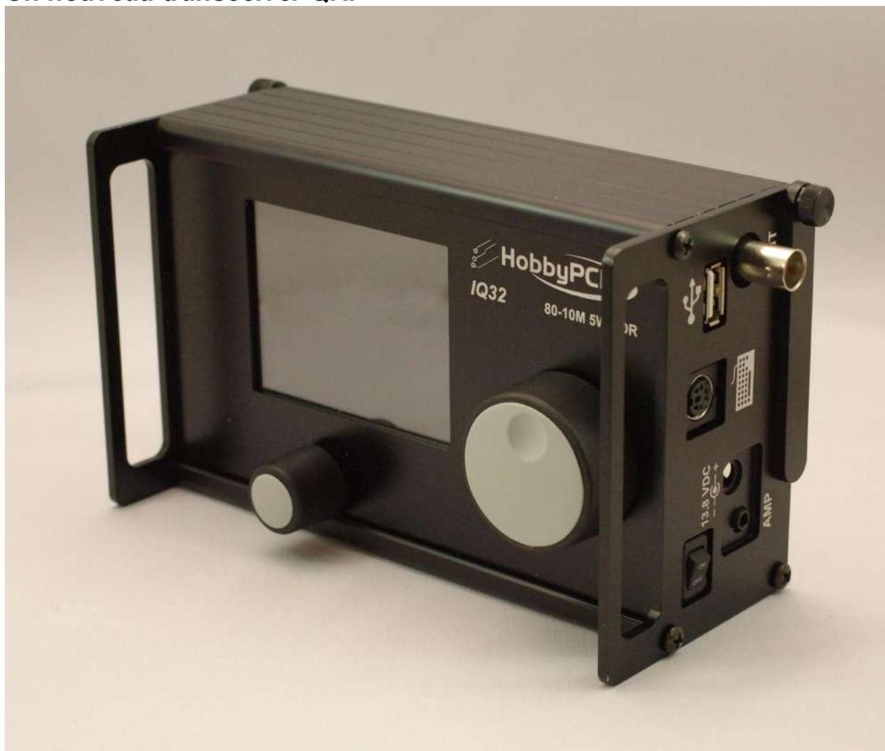
*The HobbyPCB IQ-32: A general coverage portable QRP transceiver with color touch screen*
